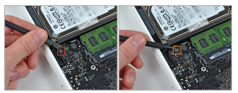
Use a spudger to pry the left speaker connector and microphone connector up off the logic board.
