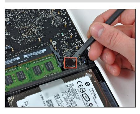
Use the flat end of a spudger to pry the hard drive cable connector up off the logic board.
