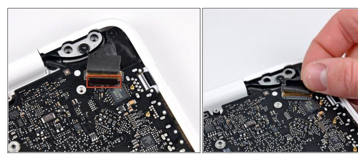
Grab the plastic pull tab secured to the display data cable lock and rotate it toward the DC-In side of the computer.
