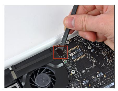
Use the flat end of a spudger to pry the AirPort/Bluetooth ribbon cable up off the logic board.
