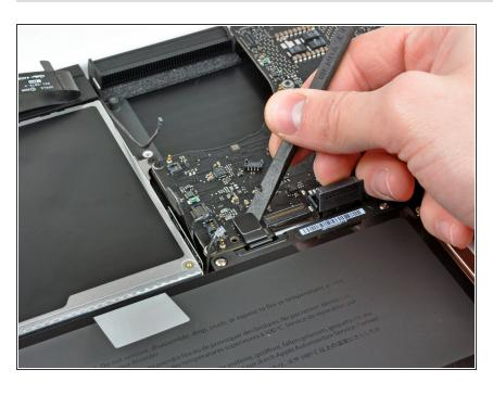
Use the flat end of a spudger to pry the trackpad ribbon cable connector up off the logic board.
