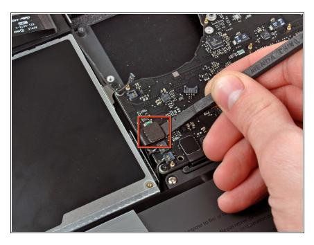
Use the flat end of a spudger to pry the optical drive connector up off the logic board.
