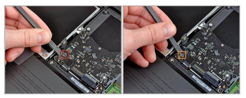
Use a spudger to pry the right speaker connector and sleep LED connector up off the logic board.
