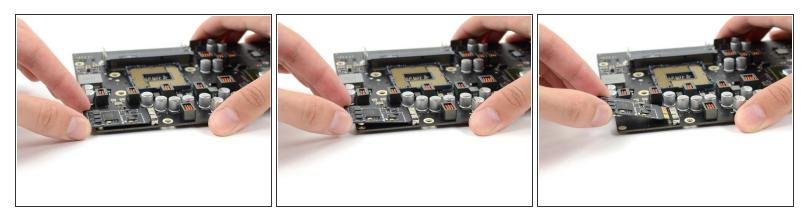
Lift the end of the AirPort/Bluetooth card slightly, and pull it straight out of its socket on the logic board.
