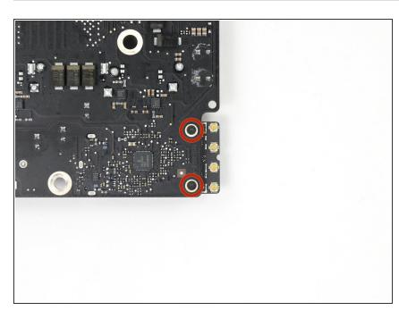
Remove the two 3.2 mm T5 screws securing the AirPort/Bluetooth card to the logic board.
