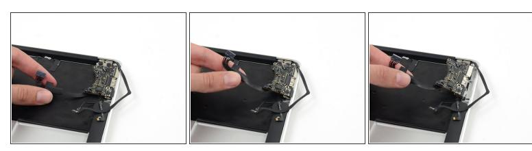
• Carefully lift the I/O board by its power cable and pull it away from the edge of the case.
