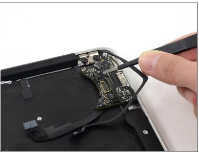
(i) If necessary, use tweezers to remove any tape covering the microphone cable ZIF connector.
