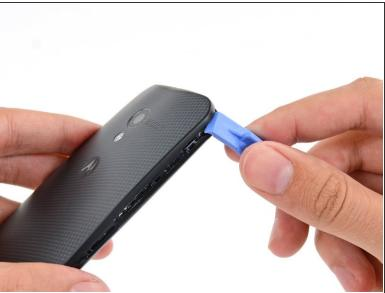
Carefully slide the plastic opening tool around the corner, freeing it from clips.
