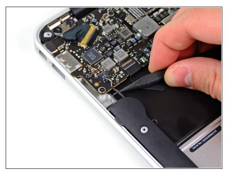
• Use the tip of a spudger to de-route the right speaker cable from the channel cut into the logic board.
