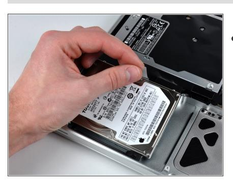
Lift the hard drive by its pull tab and pull it out of the chassis, minding the cable attaching it to the computer.
