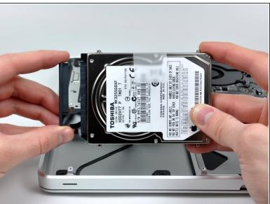
Remove the hard drive cable by pulling the hard drive straight away from the connector. Keep the connector steady. If pulled by the connector, it can be pulled too far and accidentally tear the hard drive cable.
