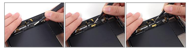
• Use a pair of tweezers to peel up the top of the rectangular piece of tape covering the bend in the front-facing camera cable.
