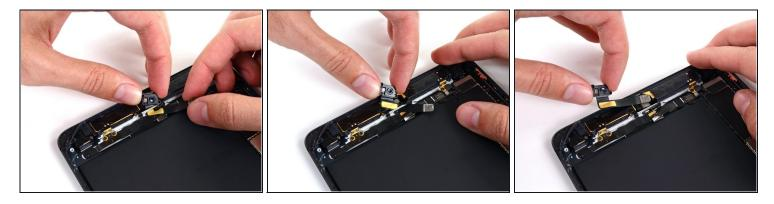
• Carefully remove the front-facing camera from the iPad, threading its cable through the slot cut near the bottom of its socket in the rear case.
