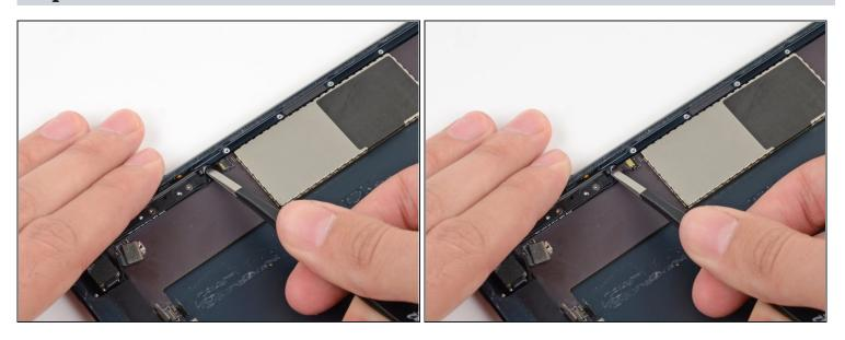
• Use tweezers to pull the button ribbon cable straight out of its ZIF socket on the logic board.
