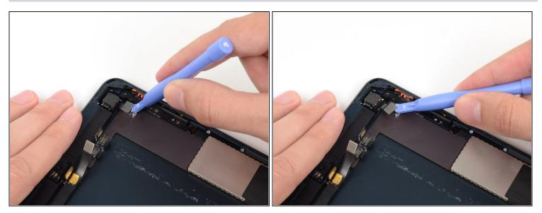
• Use a plastic opening tool to pry the rear-facing camera cable up from its socket on the logic board.
