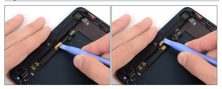
• Gently fold the front-facing camera cable up and out of the way of the logic board.
