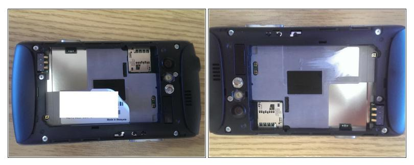
• Remove the white sticker to expose the black plastic tab that is covering the zif connector that attaches to the screen
