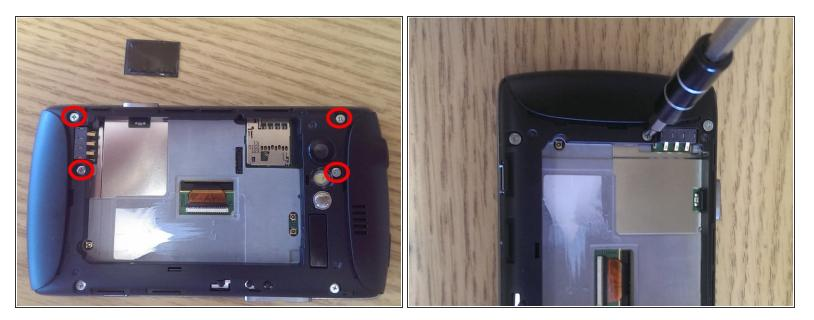
• Remove only the four screws circled in red using a Phillips #0 (PH0) screwdriver. Do not remove the others. The four circled screws hold the sliding screen down.
