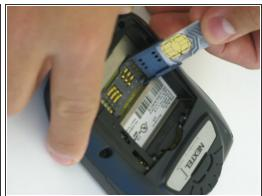
Push back on the black slot, then grab hold on top of the black slot and pull back so the SIM card and black slot pull back.
