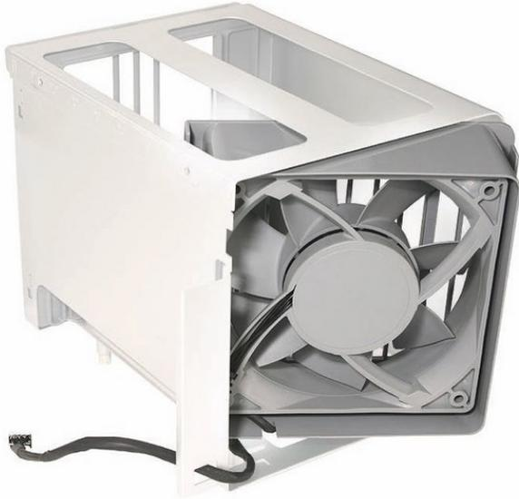
**i** Replacement Note: If you are installing a new fan in the memory cage assembly, rotate the fan into the cage as illustrated. Also note carefully the orientaton of the fan in relation to the cage.
