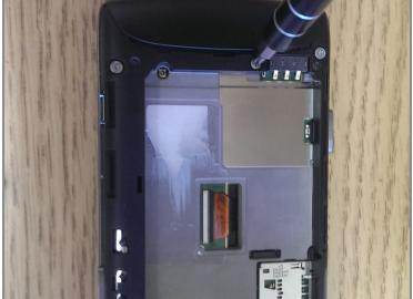
• Remove all six screws using a Phillips # 0 (PH0) screwdriver
