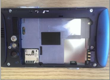
• Remove the white sticker to expose the black plastic tab that is covering the ZIF connector that is connecting the flex cable that goes between the motherboard and screen
