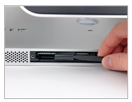
Use the sharp tip of a spudger to pull the black plastic RAM tabs out of the memory bay.
