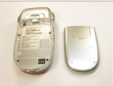
Slide the the battery release tab upwards while simultaneously lifting the back cover straight up.
