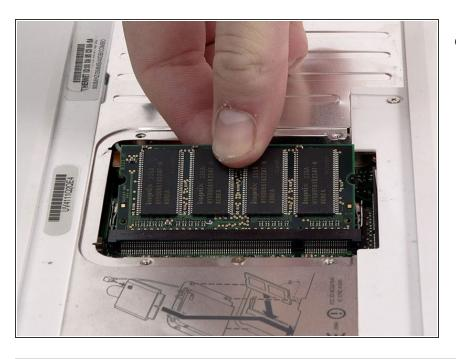
• Pull the chip directly out from its connectors.
