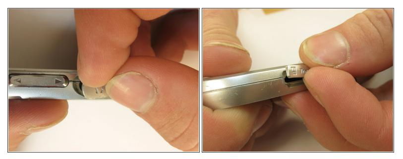
• Pull open the earphone tab and the Trans Flash tab using your fingers.
