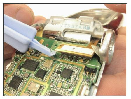
Using a plastic opening tool, disconnect the display cable from the motherboard.
