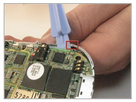
Use a plastic opening tool to pry the motherboard away from the phone housing at the tabs on both sides of the phone at the pictured location. Some force may be required.
