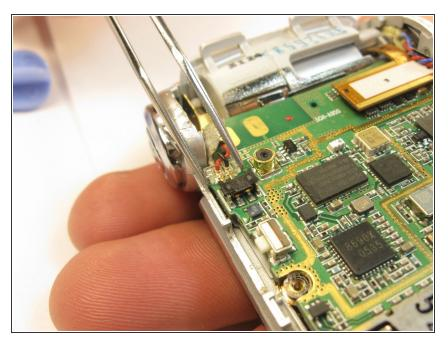
Using the tweezers, grasp the plastic connector that connects the speaker to the logic board and pull the connector off of the logic board.
