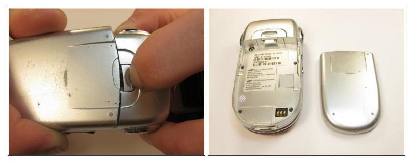
• Slide the the battery release tab upwards while simultaneously lifting the back cover straight up.
