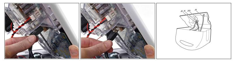
• Unplug the small USB connector from its socket (labeled J4 in the service manual).
