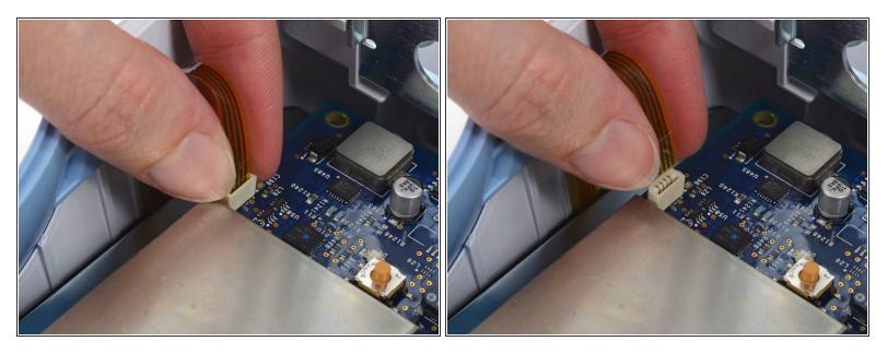
Carefully pull the LCD flex cable straight up from its socket in the motherboard (labeled J48 in the service manual).
