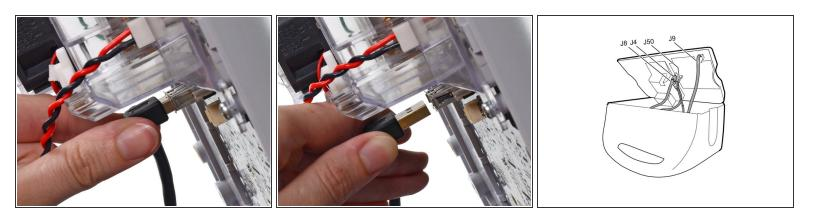
• Unplug the large USB connector from its socket (labeled J8 in the service manual).
