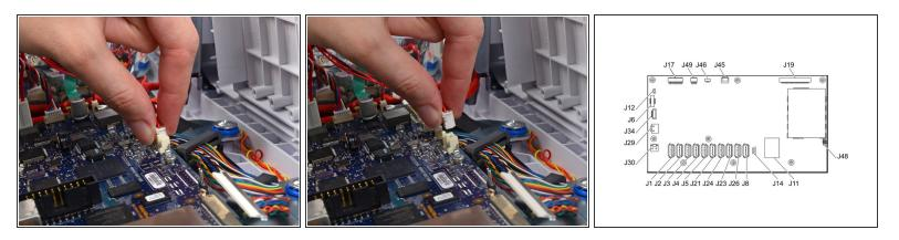
• Pinch the fan cable connector (labeled J45 in the service manual) and pull straight up to remove it from its socket.
