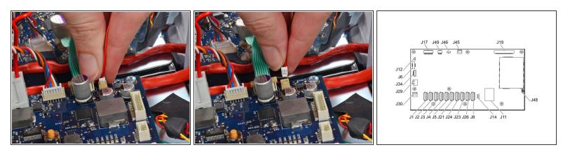
Carefully remove the speaker cable connector (labeled J12 in the service manual) from the motherboard.
