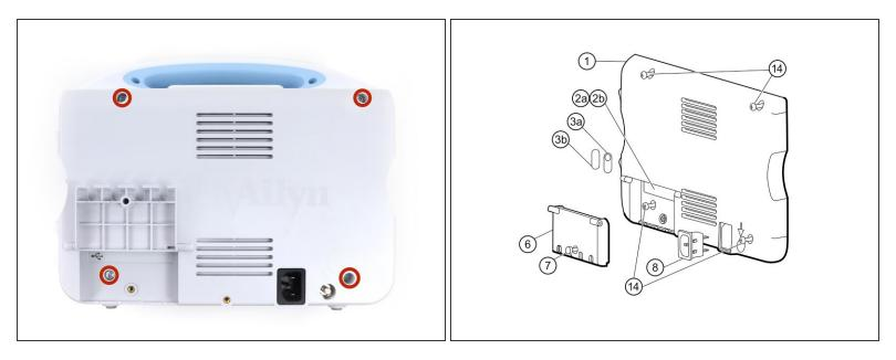
(i) Open the communications door to access the lower left-hand rear housing screw.
