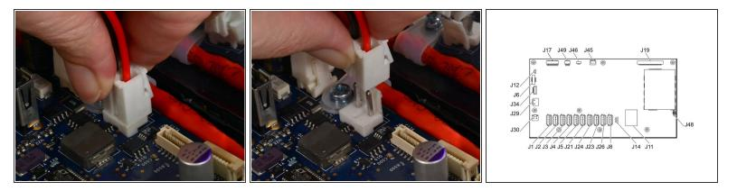
• Pinch the battery power connector and lift straight up to unclip it from its socket on the motherboard (labeled J29 in the service manual).
