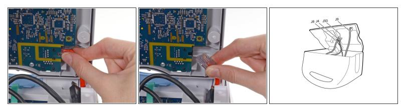
• Press the tab on the ethernet cable and unplug it from its socket (labeled J9 in the service manual).
