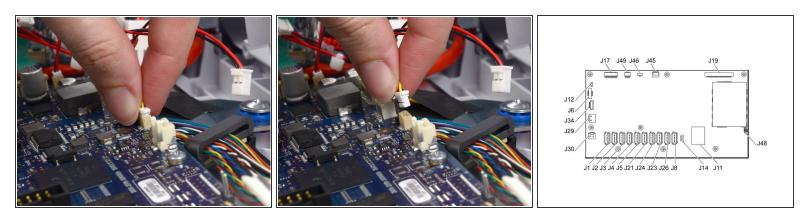
• Pull the light bar cable connector (labeled J46 in the service manual) straight up out of its socket.
