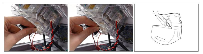
Disconnect the fan cable (labeled connector A in the service manual) from its socket in the power supply.
