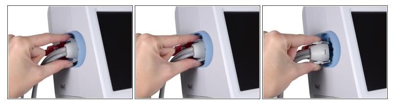
• Place your thumb and forefinger on the blood pressure (NIBP) hose connector. Squeeze the side tabs until the connector releases.
