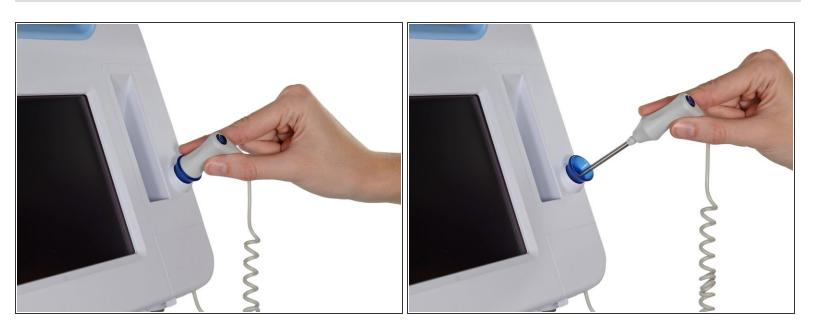
• Grasp the temperature probe and pull it up to remove it from the monitor.
