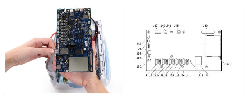
• Remove the ethernet cable connector (labeled J11 in the service manual) from the mother board.
