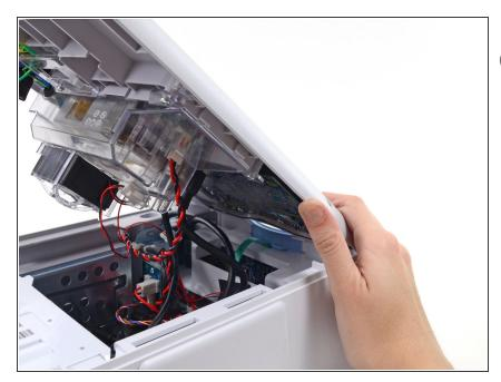
Support the rear housing while you disconnect the cables in the following steps.
