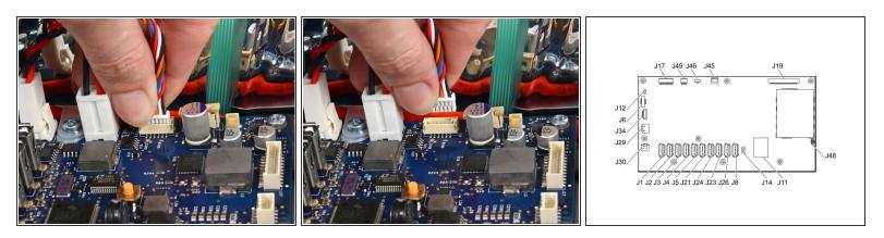
• Remove the smart-battery cable connector from its socket (labeled J34 in the service manual).
