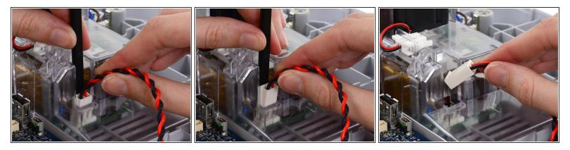
• Grasp the power supply cable firmly and lift both it and the spudger from the channel in the power supply housing to unplug the connector.
