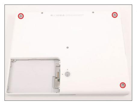
Remove the three newly-revealed Phillips screws.
