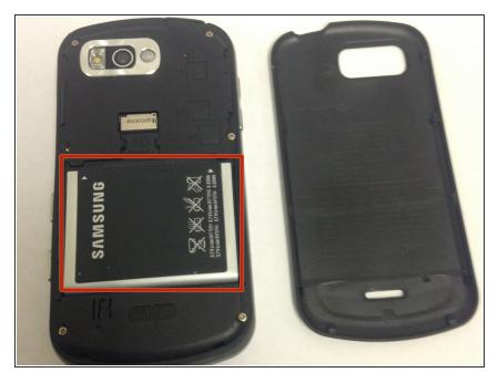
Remove the battery from the phone by pulling up on the battery edge.
