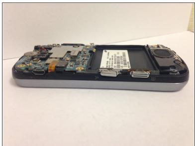
• If the camera button did not fall, carefully remove it using a pair of tweezers. At this point, you can replace the button with a new one.
