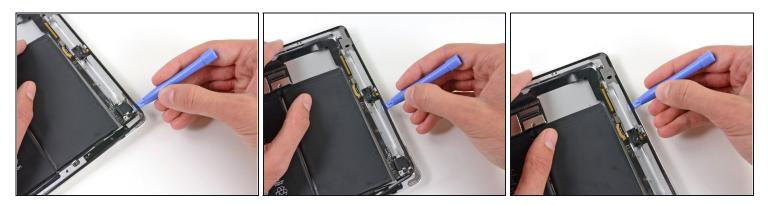
• Be mindful of the front facing camera when sliding the plastic opening tool along the top edge of the iPad.
