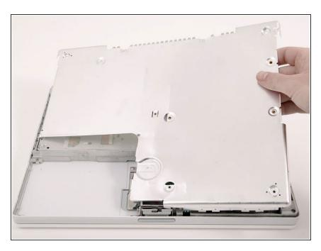
• Lift the bottom shield off.
