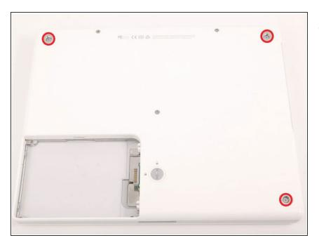
• Remove the three newly-revealed Phillips screws.
