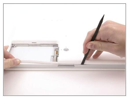
Run a spudger along the seam between the lower case and upper case on the front of the computer to free the tabs locking the lower case. Pull up on the lower case and continue to use the spudger as necessary until you hear three distinct clicks.
