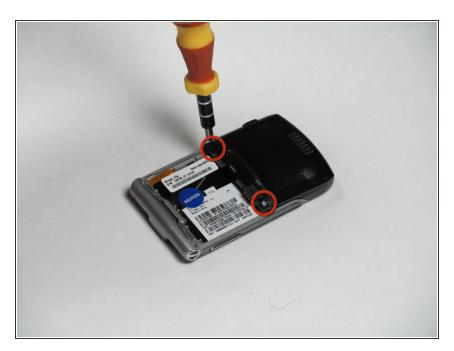
Unscrew the two screws in the back using the T6.
