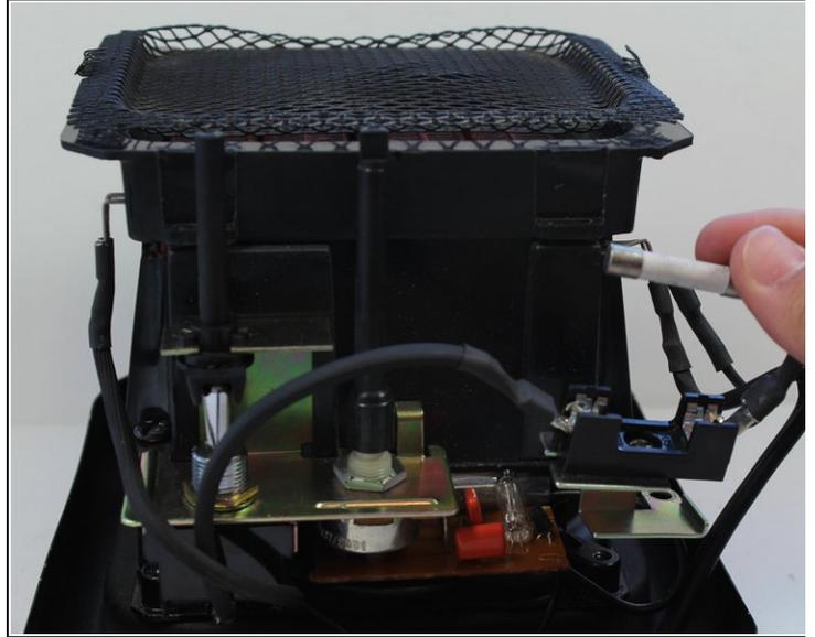
**⚠ Do not pry from the middle of the fuse because some fuses are made of glass.**
