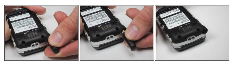
Twist the antenna off by turning it counterclockwise (relative to the picture.)
