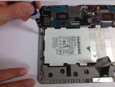
Remove the ten 3 mm Phillips #00 screws surrounding the battery.
