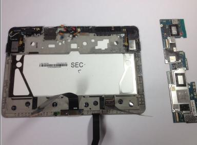
Lifting from the bottom edge, gently remove the motherboard.
