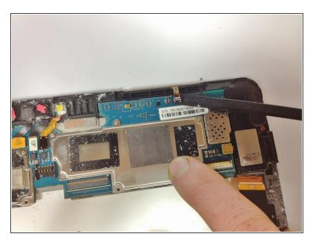
Hold down the motherboard with your finger and use a spudger to gently pry up the connection for the volume keys and power key.
