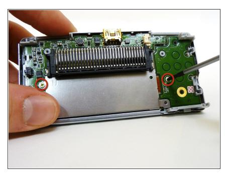
Remove the two gold Phillips #00 screws from the motherboard.
