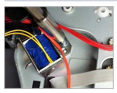
Unscrew the 10mm screw attaching the metal plate to the printer.
