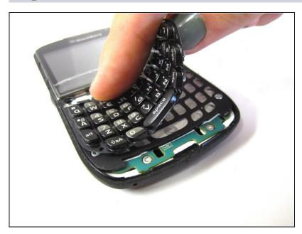
• Lift and remove the keyboard.
