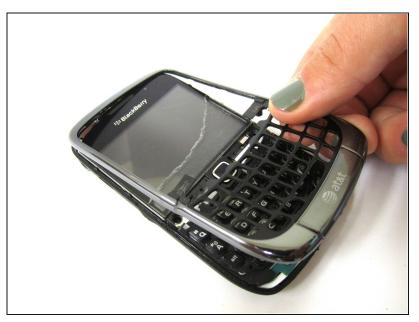
• Lift and remove the frame.
