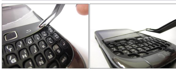
• Place the phone face up and use <u>tweezers</u> to securely grip and lift the screen upwards.
