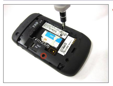
Use the T6 Torx screwdriver to unscrew the two 5mm screws highlighted.
