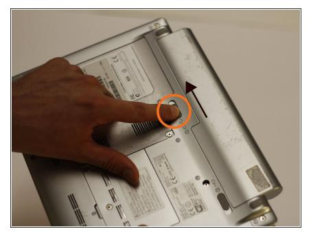
To release the battery, first slide the switch to the right.
