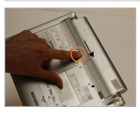
Move the switch to the left position to secure the battery and lock it in place. This ensure a strong battery connection and prevents battery from falling out. Follow this guide from beginning to end for battery removal, replacement, and cleaning.
