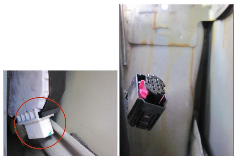
Next you want to remove the electrical cable leading to the housing. This is a black plug that fits into a white female end. The best way to do this is to squeeze the sides of the black plug, push in, and then pull it out.
