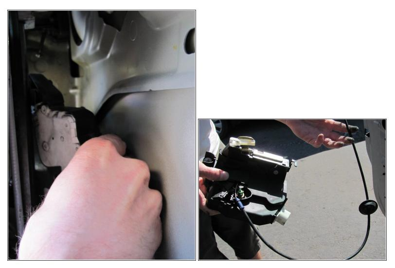
• Finally, you can take out the door lock assembly from the inside of the door. This is done by angling it slightly since it's a tight fit and almost wiggling it out between the guide rail, and the back side of the door.
