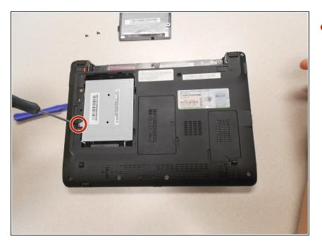
Using a Phillips #0 screwdriver, remove a third 5mm screw that holds the second cover that is directly protecting the hard drive.
