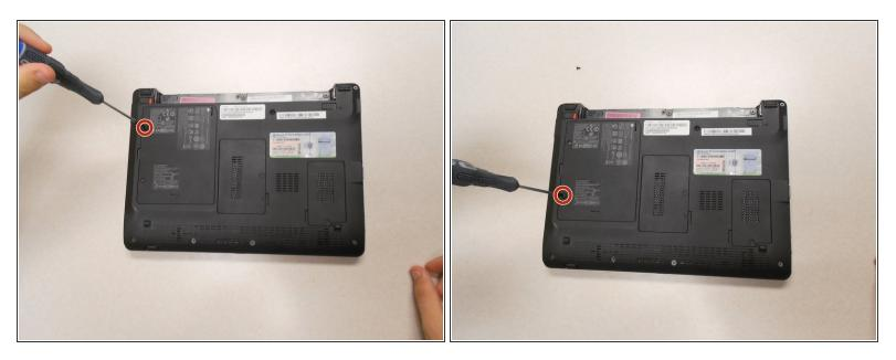
• Remove the two (2) 5mm screws holding the cover down using the Phillips #0 screwdriver.
