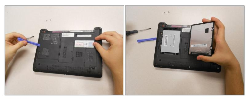
• Use a plastic opening tool to lift the cover.
