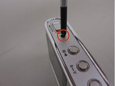
Remove the screw on each side of the device using a Phillips head screwdriver.
