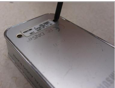
Remove the 2 screws on the back cover using a Phillips head #0 screwdriver.
