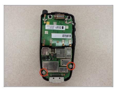
Using a Torx T8 screwdriver, remove the two circled screws by unscrewing counterclockwise.
