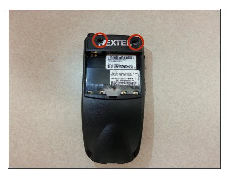
Using a Torx T8 screwdriver, remove the two screws exposed after removing the sticker by unscrewing counterclockwise.
