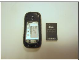
Use the plastic opener to lift, and remove, the device battery.
