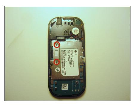
Use a screwdriver and corresponding bit to remove the two 3mm screws that attach the motherboard to the front case. Set the screws aside
