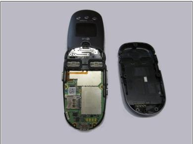
Remove the back cover completely from the phone.
