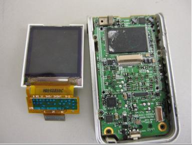
Using a plastic pry tool to flip up the lip, which connects the electric ribbon to the mother board.
