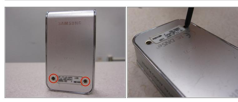
Remove the 2 screws on the back cover using a Phillips head #0 screwdriver.
