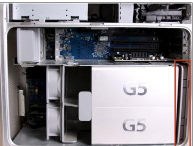
The cooling fan unit is located on the bottom right of the Apple G5 Desktop.
