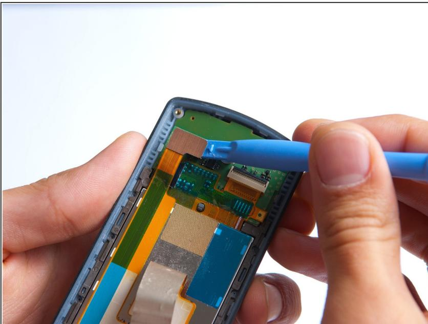
**⚠** Be very careful to not damage the keypad board when using the plastic opening tool.
