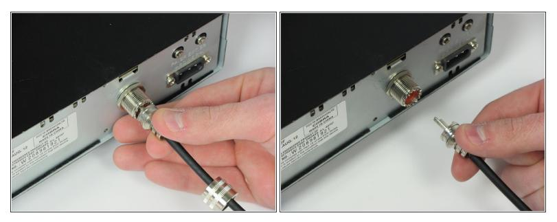
• Gently pull the antenna cable to remove it from the back of the radio.
