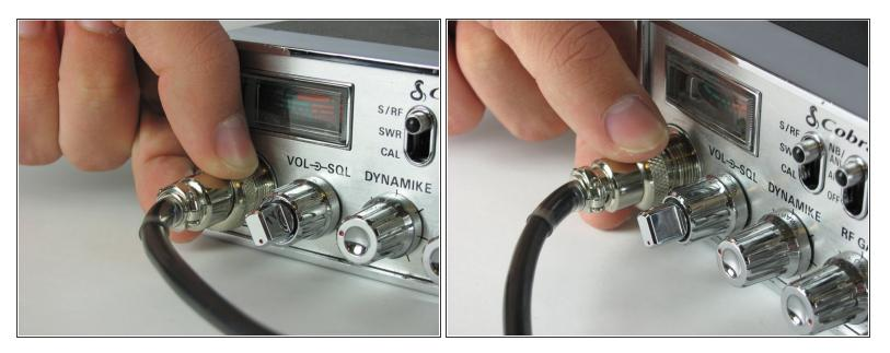
• Unscrew the cap counterclockwise on the microphone plug to disconnect the cable.
