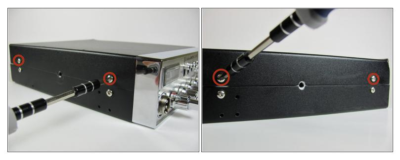
Unscrew the top four 6.0mm Phillips head screws counterclockwise on the left and right side of the device using a #1 Phillips head screwdriver.
