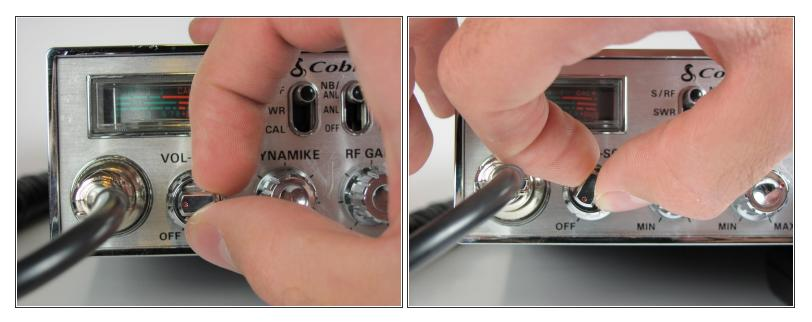
• Turn the power switch, the leftmost knob, counterclockwise to off.
