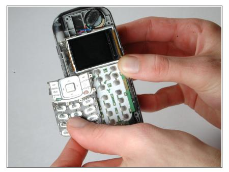
• The faceplate and keypad can now be completely removed from the phone.
