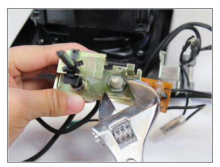
Remove the nut from the thermostat using the adjustable wrench. Place the wrench around the nut and turn it counter-clockwise. Remove the thermostat/circuit board assembly from the gold metal bracket.
