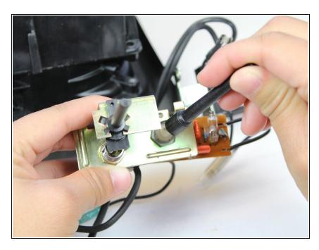
Pull off the black thermostat extension by pulling up. This should require very little force and should come apart easily.
