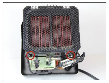
Remove the two 10 mm Phillips screws using a #2 Phillips screw driver. One attaches the gold metal bracket to the heater coil housing and the other attaches the fuse holder to heater coil housing.
