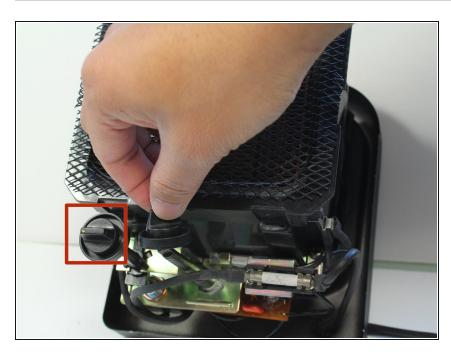
Remove the two dial caps from the two switches by lifting them up.
