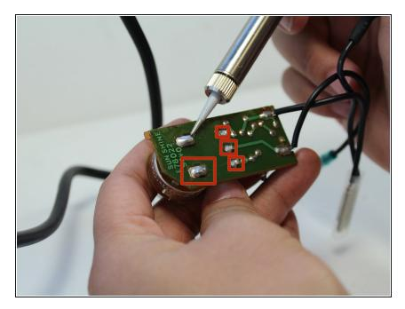
Use the soldering iron to remove solder from the five points connecting the thermostat to the circuit board. Pull the thermostat away from the circuit board.
