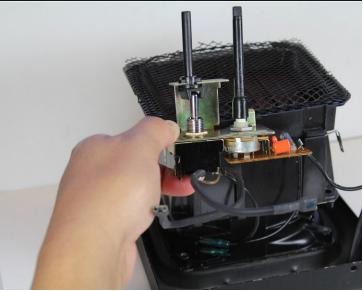
Grab the Switch and Circuit Board Assembly with one hand and slide it up. You will need to wiggle it to break it loose. While wiggling it, slide it up until it is clear of the plastic rails.
