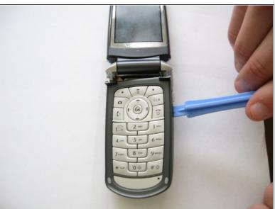
Use the spudger to remove the keyboard plate.
