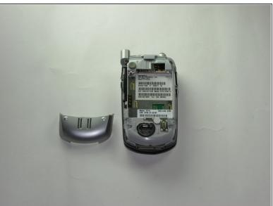
Use the spudger to remove the bottom plate.
