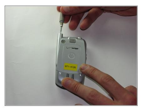
Unscrew the antenna with a clockwise motion and pull to remove the antenna.
