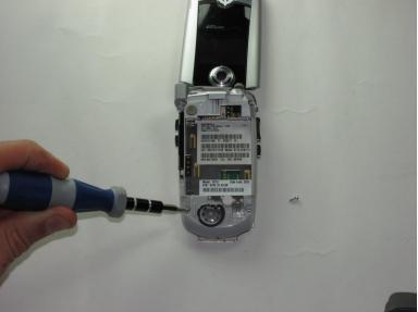
Unscrew the bottom two screws with the T6 screwdriver.
