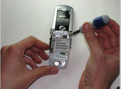
Remove the screws under the antenna and to the right side of the phone with the T6 Torx screwdriver.
