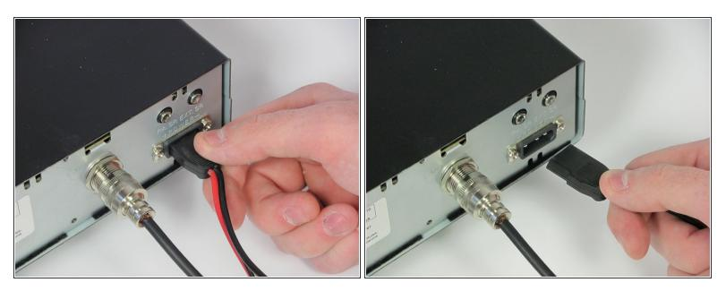
• Turn the device around and firmly pull the power cable plug to remove it from the radio.
