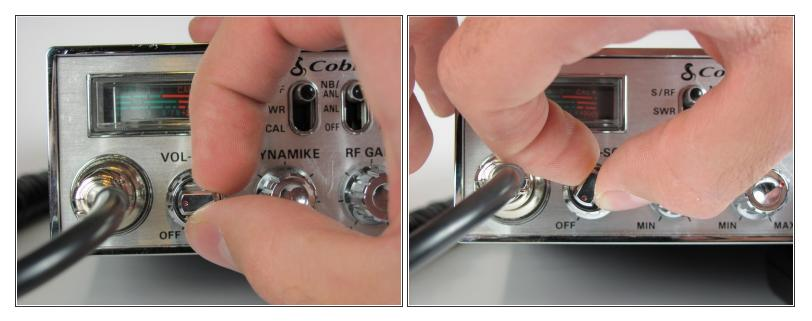
• Turn the power switch, the leftmost knob, counterclockwise to off.
