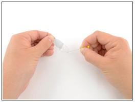
• Using your fingernail, or a pin, peel the backing off the tenacious tape, so that you only have the clear sticky layer.
