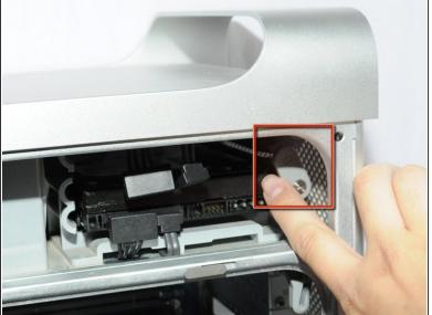
Rotate up plastic tab labeled "B" on the right hand side of hard drive.
