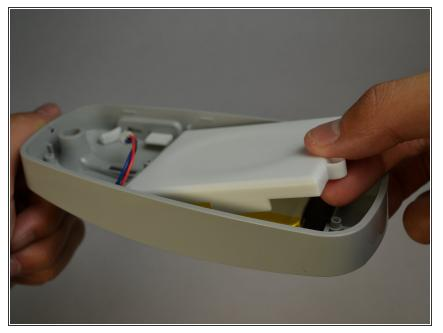
• Gently pull up the battery case out of the tabs and pull the case out.
