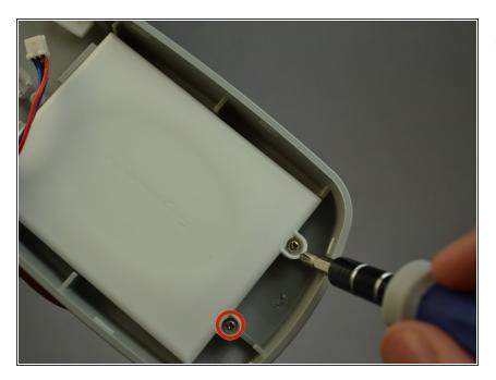
• Remove the two 2mm screws from the battery case.
