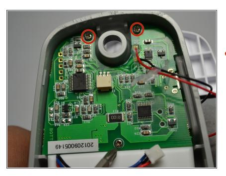
Unscrew the three 2mm screws holding the circuit board down using a Phillips #1 screwdriver.
