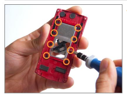
Unscrew the eight Phillips #000 (1mm) screws on the back side of where the sliding mechanism is located.
