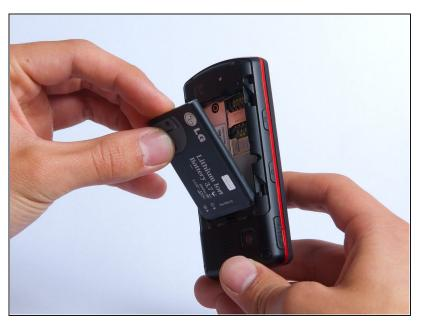
• Lift and remove the battery.
