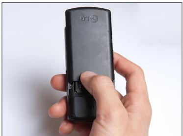
On the back of the phone, place your thumb on the three raised bumps and slide the back cover upward.
