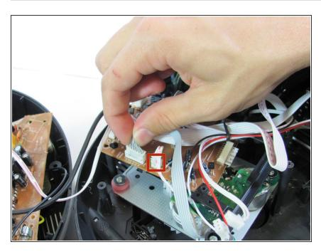
Remove the two white ribbon cables attached to white plastic connectors from the circuit board by pinching the tabs with your hands and pulling outward on the connector.
