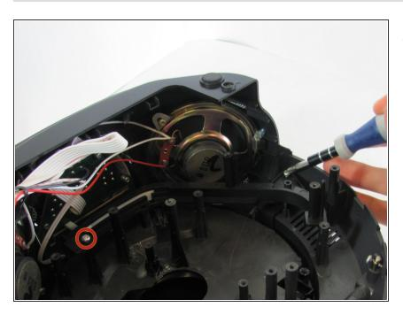
With a Phillips #2 screwdriver, remove the two 3mm screws from the black plastic tuner frame.
