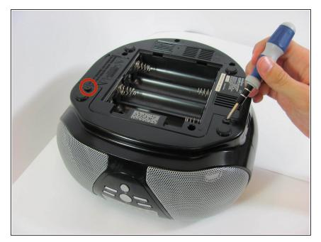
With a Phillips #2 screwdriver, remove two 2mm screws.
