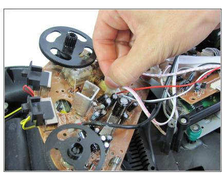
On the brown side of the quarter circle circuit board, remove the two white ribbon cables with pink stripes attached to a plastic connector. To do this, pinch the tabs with your hands while pulling outward on the connector.
