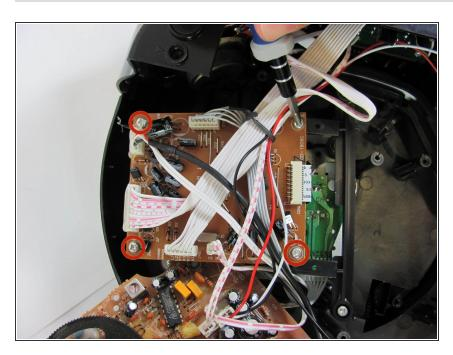
With a Phillips #2 screwdriver, remove four 6mm screws from the rectangular circuit board.
