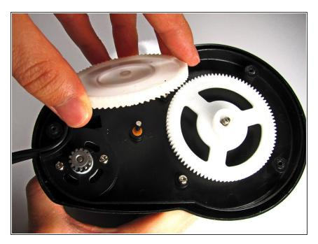
Remove the smaller white gear by lifting it up with your hand.
