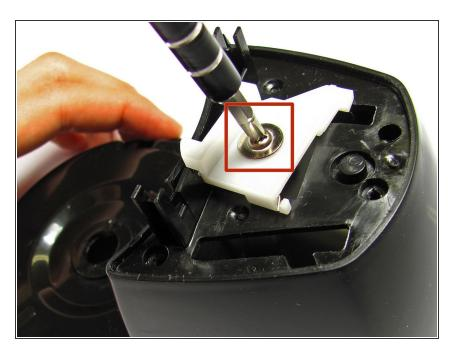
Use the Phillips #2 screwdriver to remove one 9.53-mm screw.
