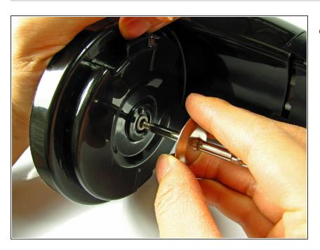
Use your hand to firmly pull the blade-shaft from the base.
