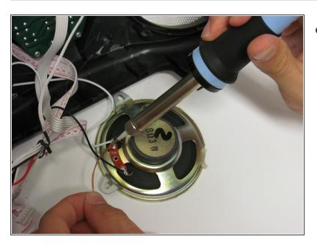
Remove the solder from the two black and white wires connected to the speaker.
