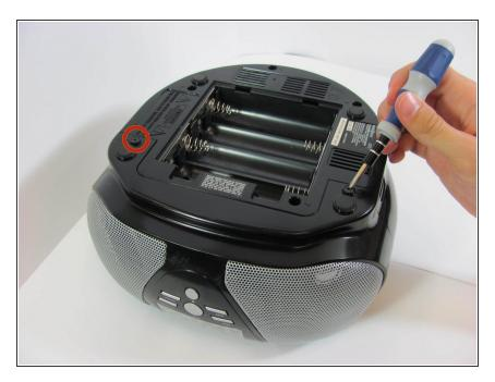
With a Phillips #2 screwdriver, remove two 2mm screws.
